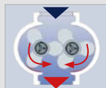
Conveying to discharge side
